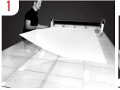
Place the substrate on the table. Align adhesive media on top of the substrate.
