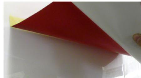
4. Hold the graphic smooth and taut, away from the application surface with one hand and squeegee horizontally from the centre towards the outer edges. Continue squeegeeing, using firm overlapping strokes from the centre out, working away from the starting point. Pull the liner back as necessary.
