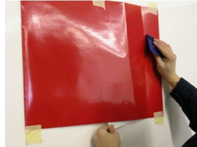
3. The tape will help to hold the graphic smooth and taut, away from the application surface, however it is helpful to use one hand to help keep tension on the film. With the other hand squeegee vertically from the centre towards the outer edges. Continue squeegeeing, using firm overlapping strokes from the centre out, working away from the starting point. Pull the liner back as necessary.
