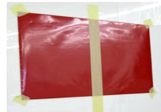
3. Choose which of the graphic you would like to apply first (left or right). Separate this side of the graphic from the liner and remove this section of the liner by cutting it with a scissors or razor knife.
