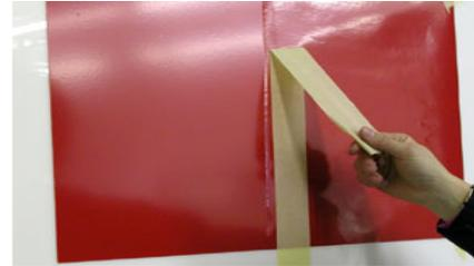
6. Reach behind the graphic and carefully pull the liner back several inches to expose the adhesive.
