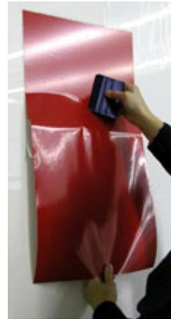
8. Re-squeegee the entire graphic using very firm squeegee pressure, including all edges. Puncture any air bubbles with a straight pin and re-squeegee from the edge of the bubble towards the puncture.
