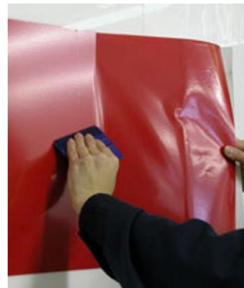
8. Re-squeegee the entire graphic using very firm squeegee pressure, including all edges. Puncture any air bubbles with a straight pin and re-squeegee from the edge of the bubble towards the puncture.
