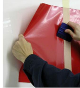
5. Once the first side is applied remove the hinge so that the opposite side can be applied.
